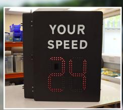
Prompting drivers when exceeding the speed limit, or highlighting the legal limit of a given area are both proven methods of speed reduction.
