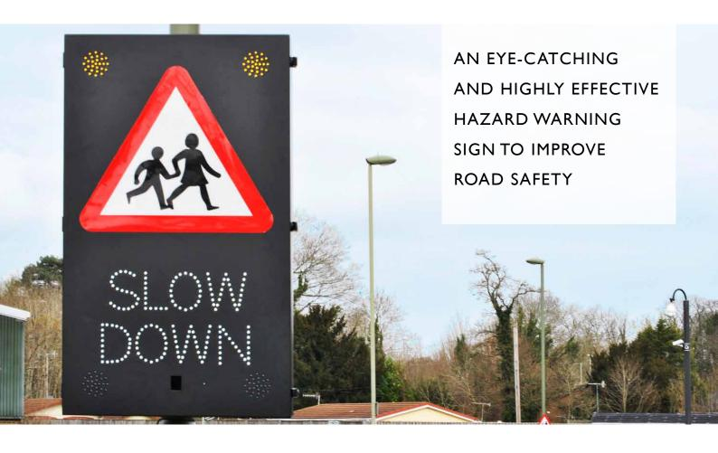
Messagemaker Displays versatile and innovative solution for hazard warning and traffic calming; the Vehicle Activated Warning Sign.
