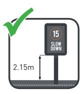
2.15m minimum between the base of the sign and the ground
