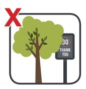
Avoid placing underneath overhanging trees/hedges, especially if using solar panels
