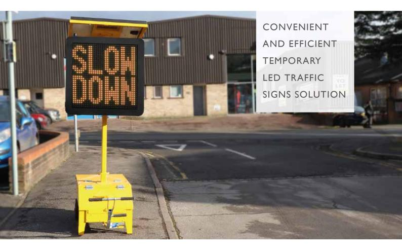
Variable Message Signs (VMS) and Vehicle Activated Speed Signs (VAS) are becoming increasingly popular on UK highways due to their energy-efficiency, intelligent technology and ease of use.
