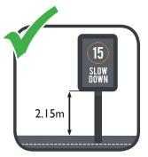
2.15m minimum air space between the base of the sign and the ground
